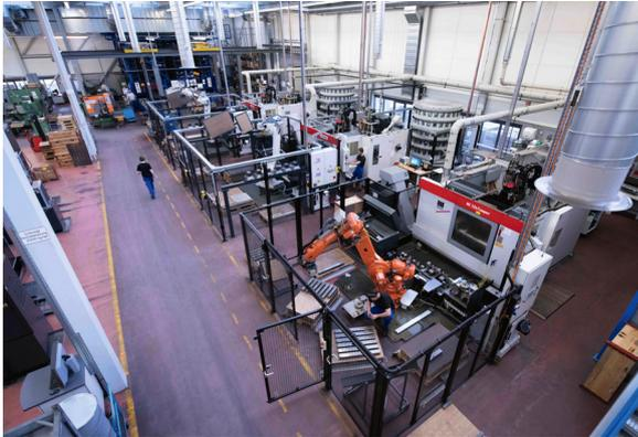
The highly automated production with cutting edge 5-axis machining centers is located in-house at Bucher Hydraulics.
